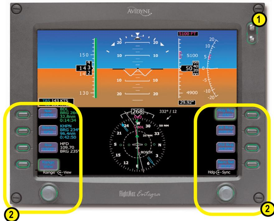
**1. Brightness Control (BRT/DIM)-** Controls display brightness. Power-on default is 75% brightness.
