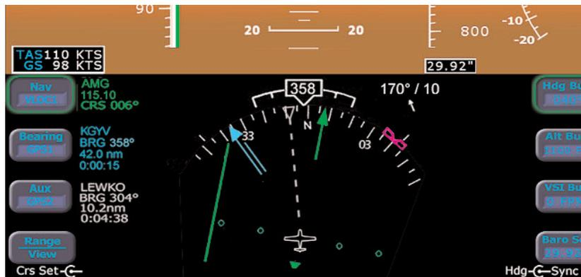
The wind vector on the HSI is very useful in any phase of flight where winds aloft should be taken into account. A combination of the wind vector and projected track line can be used to your advantage in navigation tasks. A very useful technique is to align the projected track line with the desired course. This will take the guess work out of determining proper crab angles for wind corrections.
