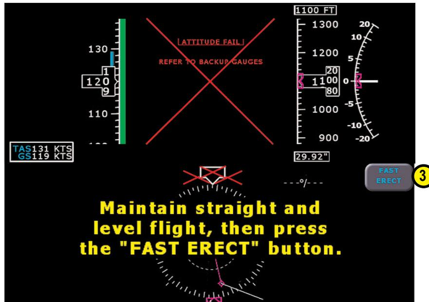
In the unlikely event of a recoverable attitude data failure, all normal button labels will be removed and:
