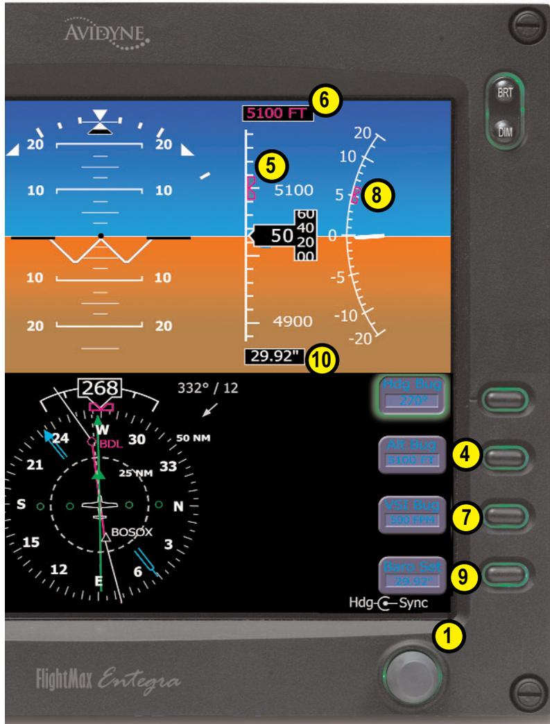
**4. Altitude Bug Button (Alt Bug)-** When selected, allows the right knob to control the position of the altitude bug and the autopilot altitude preselect value. The range of values is the same as the altitude tape (-1,000 feet to 25,000 feet). The Alt Bug has three resolution setting modes: 1,000 ft, 100 ft, and 10 ft modes.
