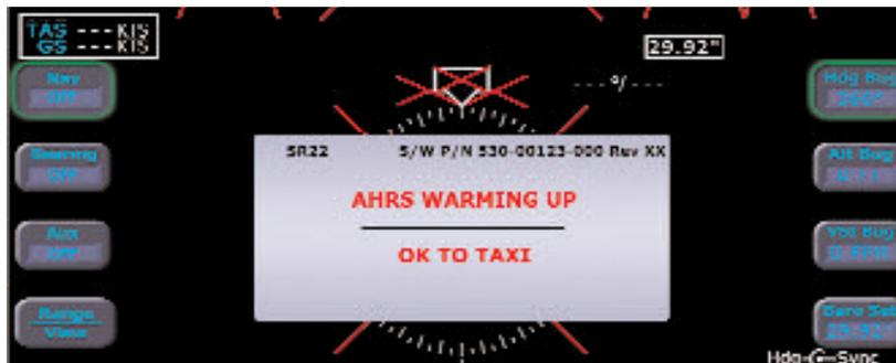
When the system is approaching its final alignment phase, the message changes to the one depicted in the next figure, indicating that the pilot should bring the aircraft to a stop as soon as it is practical. This will be presented for several seconds, even if the aircraft is stationary.
