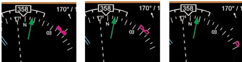
The bug is solid when coupled with the autopilot, and hollow when not coupled. The heading bug is positioned at the appropriate side of the tape and remains in partial view when "arc view" is selected and the selected heading bug value is outside the current compass rose field of view.
