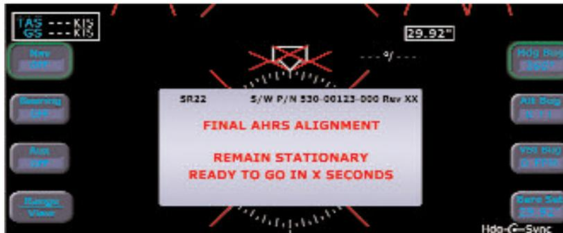
In the event that the AHRS is unable to complete its alignment, the following display is presented. If this occurs, wait approximately an extra two minutes in this state. If the system picks back up on the alignment, a nominal PFD will result. If the display does not clear itself, contact a service center and provide the displayed error code.
