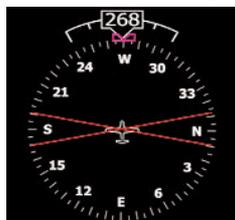
Until a flight plan is activated in GPS/Nav 1, the HSI will show a red "X" in place of the CDI.
