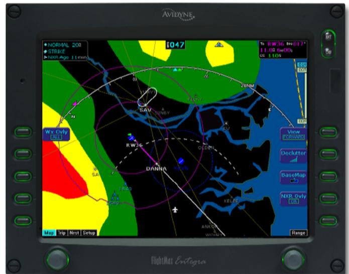
The FlightMax Entegra primary flight display (PFD) and multi-function display (MFD) are designed to provide pilots with all the information needed to manage the aircraft and safely determine routes, speeds, as well as proximity to adverse weather conditions, terrain, obstacles, and other aircraft.
