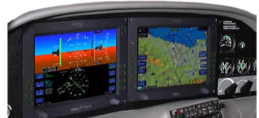
FlightMax Entegra's fully-integrated instrumentation and built-in datalink provide light general aviation with its first integrated flight deck.
